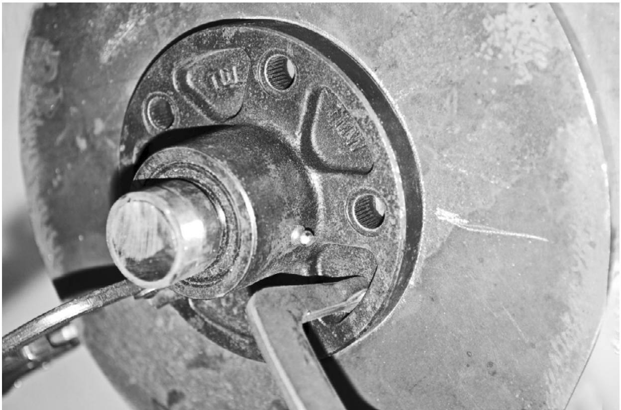
Figure 3 Hub/Spindle Assembly (Flange “Side-Up”) Clamped to Hemisphere’s Top Plate
