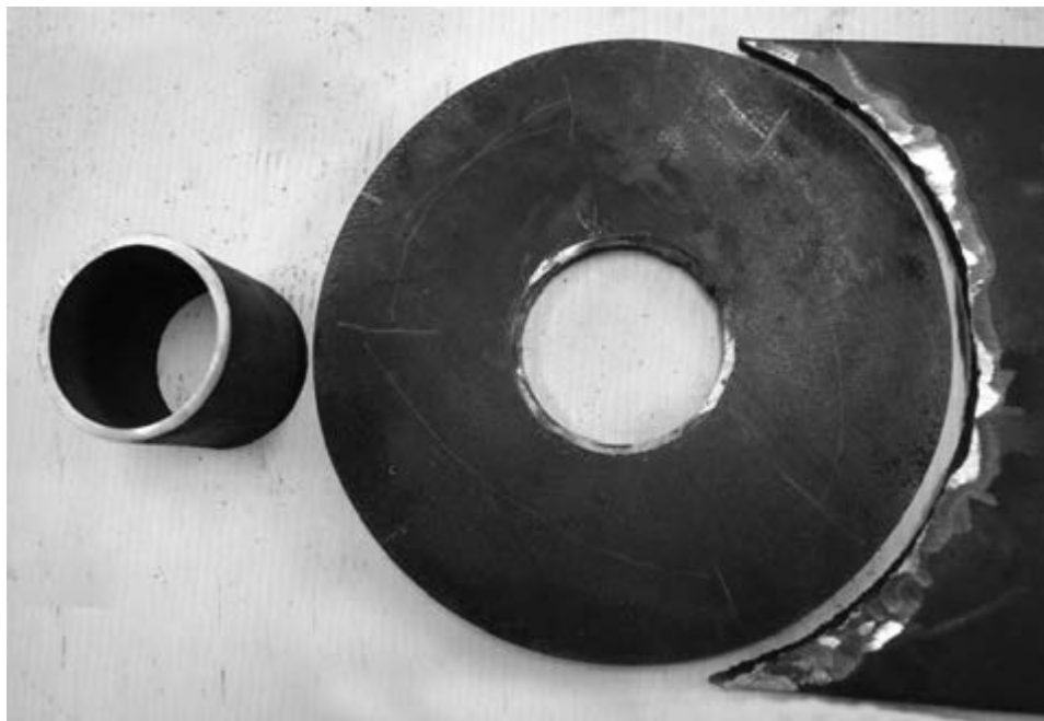
Figure 2 Hemisphere's \frac{1}{2} " Top Plate Top and Hub/Spindle Cup
