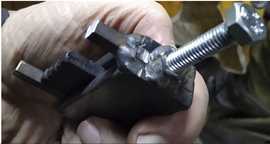
Photo 6: Welding the Nut for the Clamp Bolt
