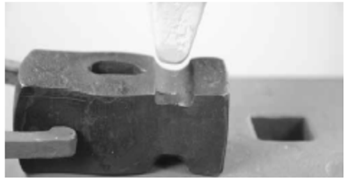
Work the top and bottom surfaces. The sides have been pushed out by the punch and are not flat
