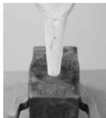
Working from one side, punch half way through the bar. Turn the bar end-for-end between blows Aim to join the two holes in the center of the bar.
