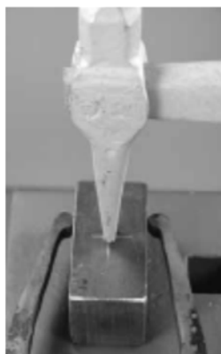
Working from one side, punch half way through the bar. Turn the bar end-for-end between blows Aim to join the two holes in the center of the bar.
