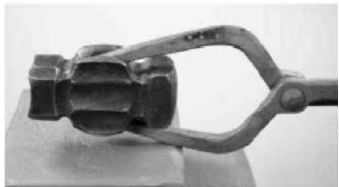
Tongs gripping the stock with the tips of the jaws in the hammer eye
