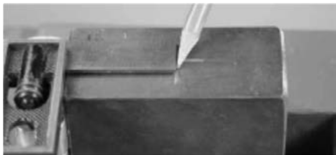
Using a set of Dog-leg dividers or an adjustable square, find the center of the block
