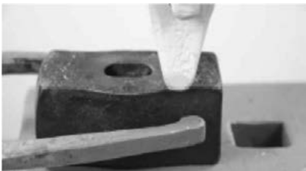
Being flat, the stock will sit on the anvil as you create a fullered groove defining the body and the faces
