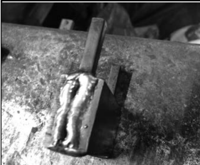
Photo 2: Welding the End Pieces
