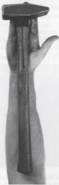
The late Francis Whitaker's method of fitting handle length to the smith.
