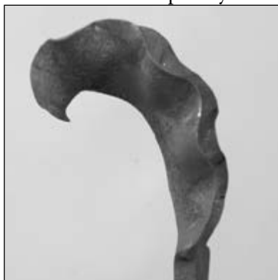
Fig. 12 The leaf, forged and formed
