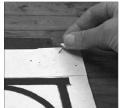
Fig. 3 Pin or tape the drawing down over the rusty tin-plate
