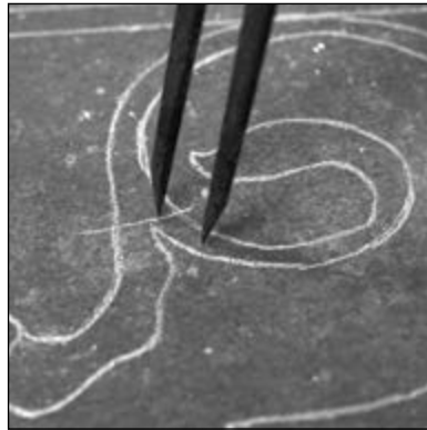
Fig. 6 Step out from that datum point to the tip of leaf and scroll
