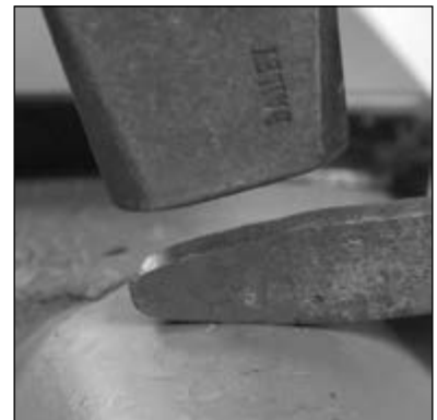
Fig. 10 Draw a short, rounded taper to the bar. Maintain stock thickness
