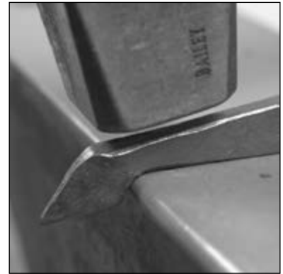
Fig. 7 Forge the end to the beveled leaf scroll
