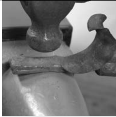
Fig. 15 Weld on the back and face of the anvil
