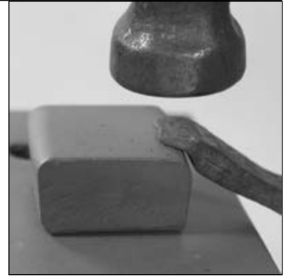
Fig. 16 Form the scarf with the step on the leaf side
