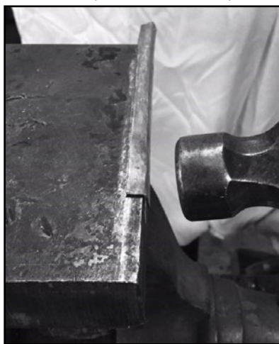
Left: Jig for making angle iron under treadle hammer with customized chisel peen for this step. Middle: Developing sharp crease carefully against sharp edge using glancing blows. Right: Curved square stock to shape ribs.
