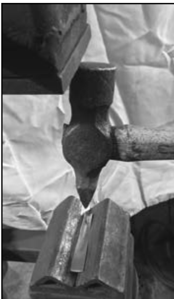
Left: Jig for making angle iron under treadle hammer with customized chisel peen for this step. Middle: Developing sharp crease carefully against sharp edge using glancing blows. Right: Curved square stock to shape ribs.
