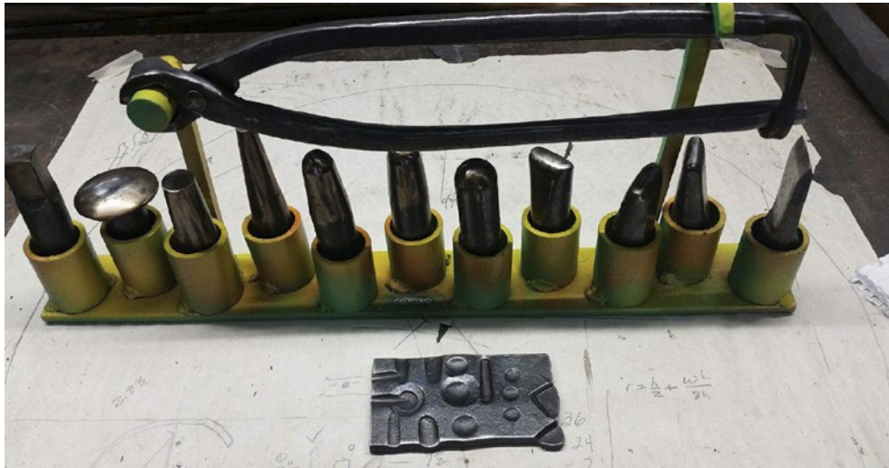
Decorative Punch Set by Gerald Franklin - Hot cut is S7. The other punches are 1045 water hardened and tempered at 425 degrees for 2 hours.
