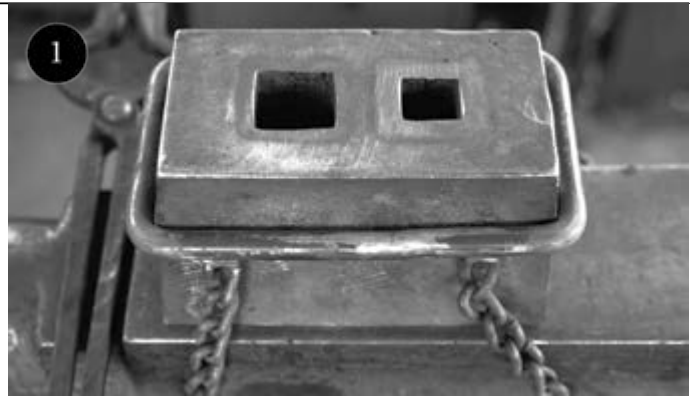
The swage block bolted down, with tensioning chains passing under the throat and heel of the anvil
