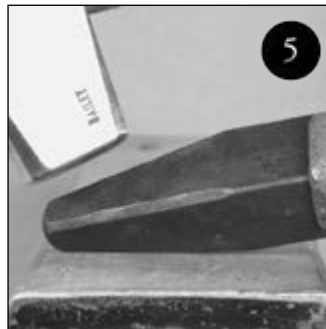
Chamfering the edges now will protect the taper from the fire as you take a high heat
