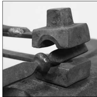
A clam shell that makes my closed die tooling to complete the welded collar
