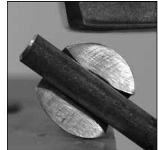
Welding a collar onto a length of round bar is a two step process, first weld the middle of the collar and then weld the edges of the collar at the edge of the anvil
