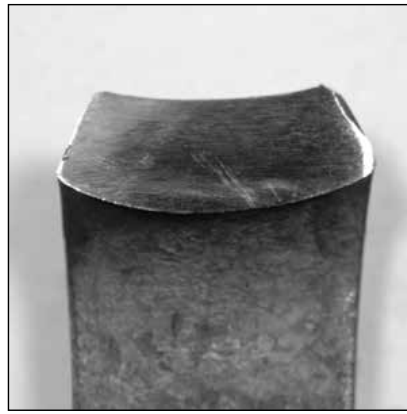
A flat bar bent the easy way has deflected the edges away from the bend
