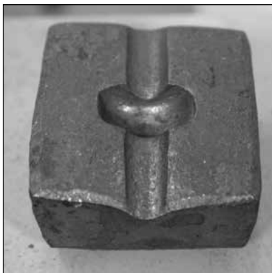
The result of driving in the half-round end of the flat bar to make the recess for the collar material
