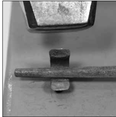
A flat bar bent the easy way has deflected the edges away from the bend
