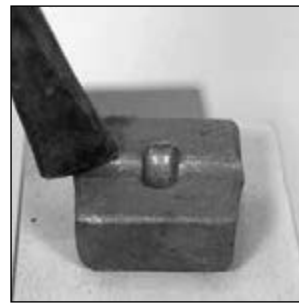
Using a hand-held fuller to let-in the recess for the cone material of the blank
