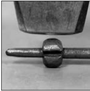
Welding a collar onto a rose stem to form the rose hip
