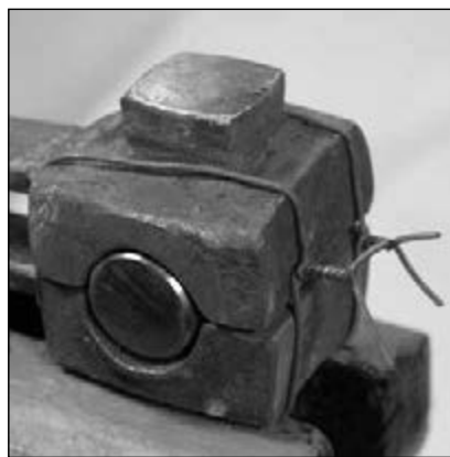
The blank wired in place to keep both sides in alignment as the staple is welded in place
