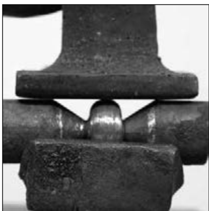
Using a flatter to deliver an even blow will help prevent damage to the blank
