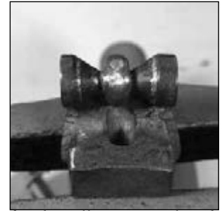
Left: cleaning up the recess for the collar material and right: the result with the blank shown for comparison
