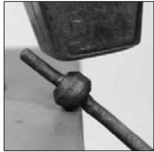
Welding a collar onto a rose stem to form the rose hip
