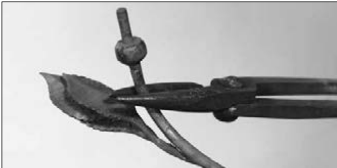
A welded collar on round stock forming the hip of a rose at the base of the flower
