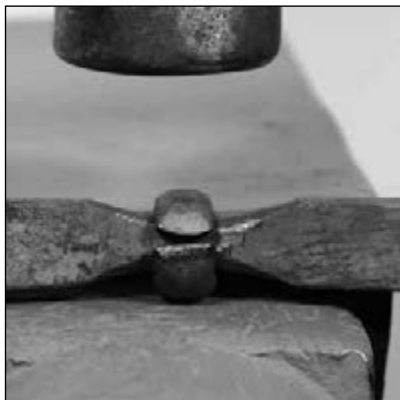
A collar wrapped around the necked-in rectangular bar of the center style of the grille
