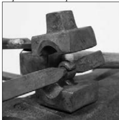
My hammer is keeping the dies apart as I place the hot material between the clam shell tooling
