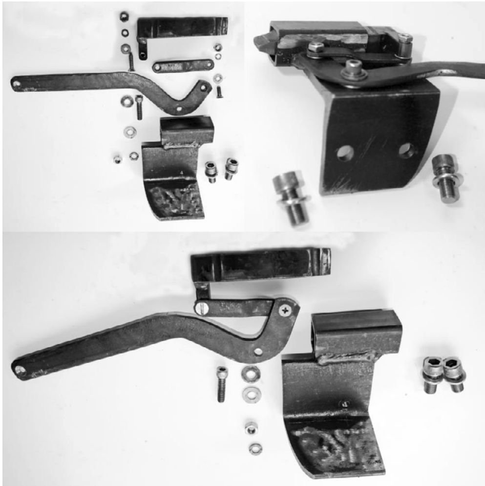
Figure 8 Table Lock Elements and Assembly
