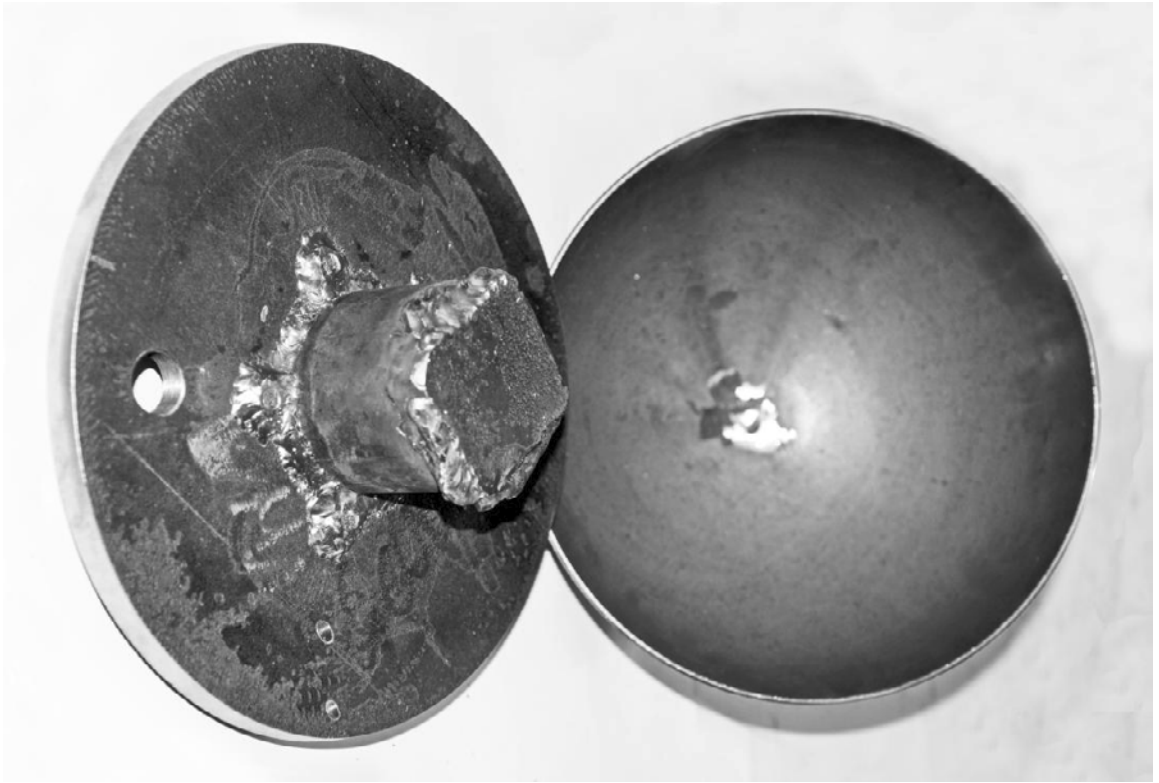
Figure 10 Assembling Hemispherical Base with the Completely Fabricated Top Plate
