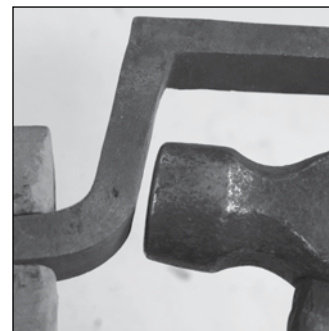
Fig. 15. Extend the flat down to level with the mark and then move to the anvil
