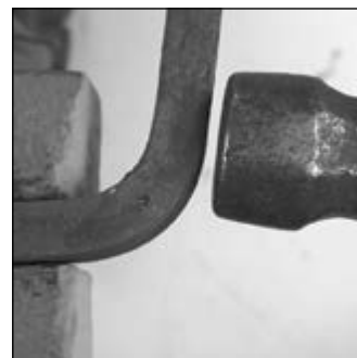
Fig. 8. Start the center of the hammer at the bottom of the straight section of arm
