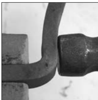
Fig. 2. Hammer not aligned with arm. The toe of the hammer is causing a bend in the bar
