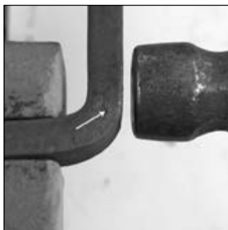
Fig. 9. Extend the flat to just about level with the center-punch mark
