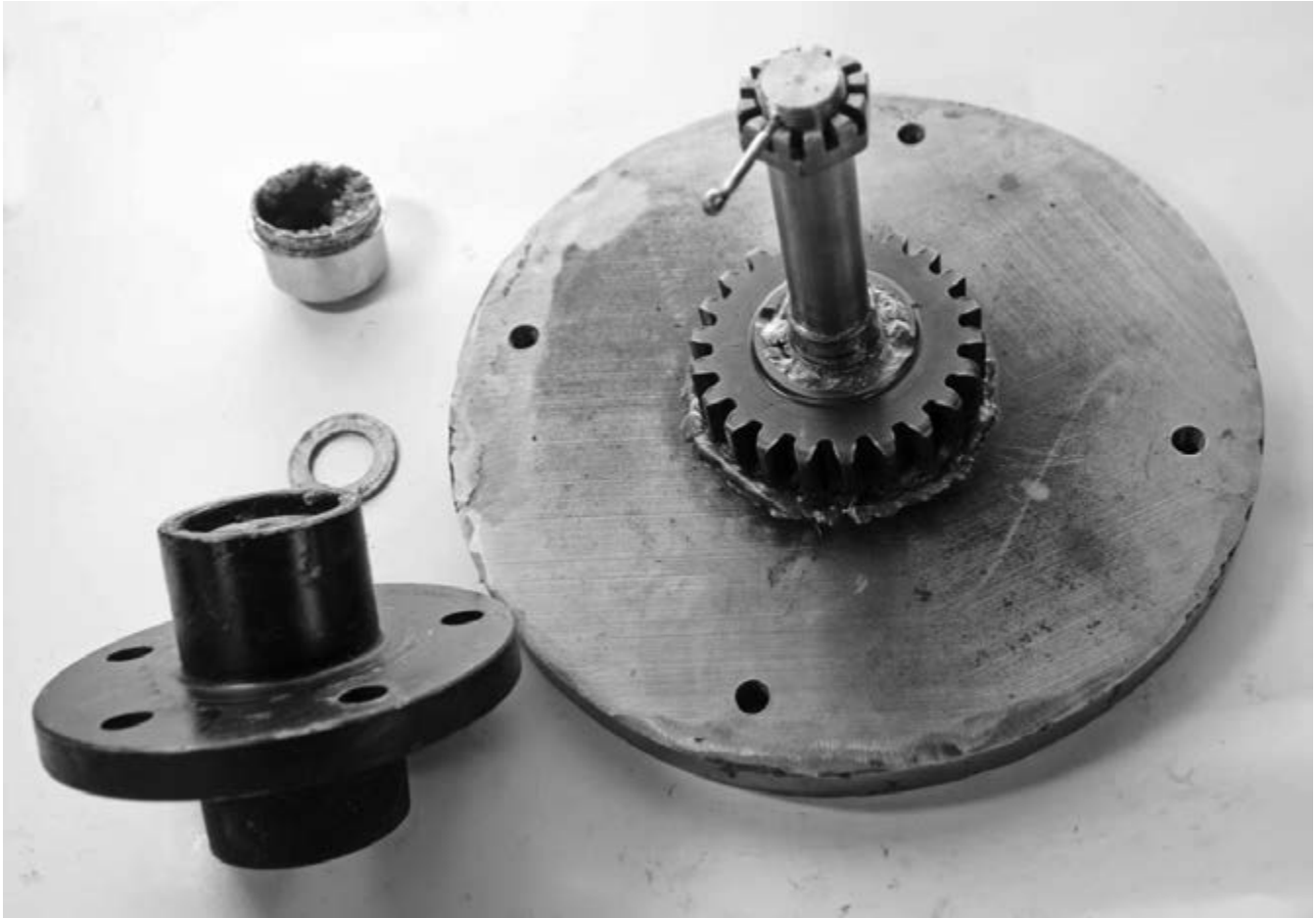
Figure 6 Disassembled Hub/Spindle; Welded Spindle, Spur Gear and Table Platform
