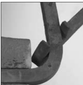
Fig. 1. The bend has been taken too far. It is past the 90° position
