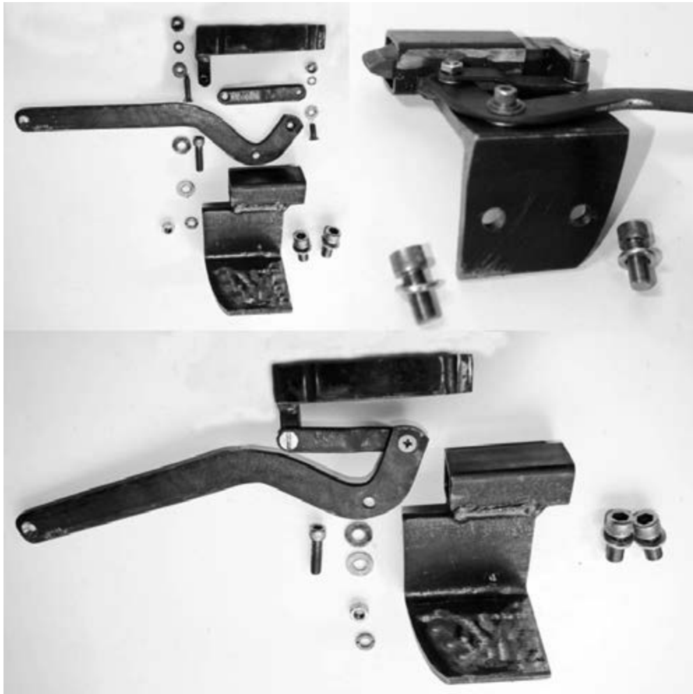
Figure 8 Table Lock Elements and Assembly
