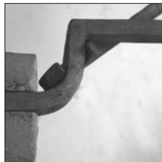
Fig. 14. The second bend can be made accurately at the vise
