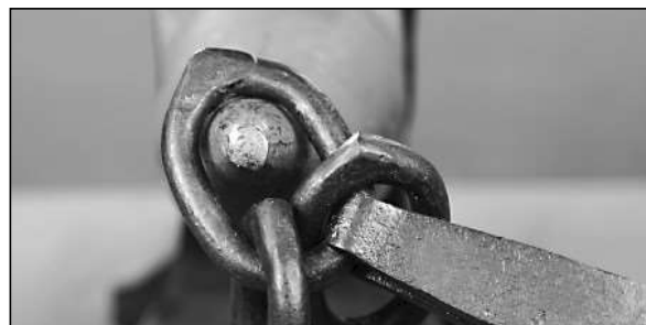
I try to keep one link either side of the tong jaws as I continue to weld on the bick.
