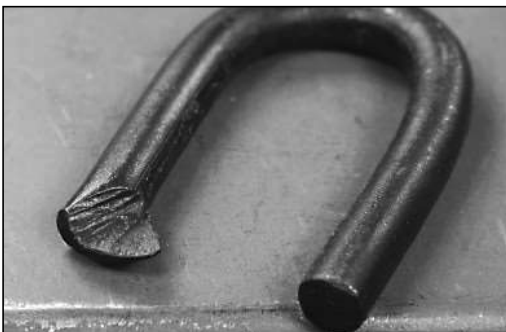
A chain-step-scarf on one end of the bar.
