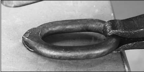
Weld on the flat face of the anvil first.
