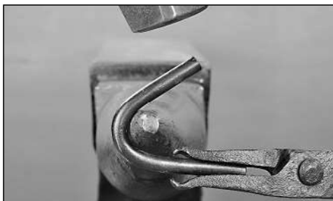
Keep an eye on the length of the arms. Try to keep them of equal length. Stop if they get out-of-whack.
