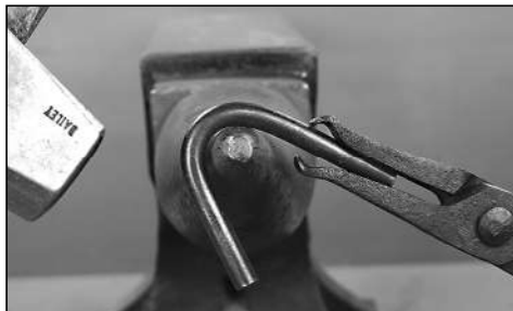
Get as far as you can, working from the top, and then turn the link over.
