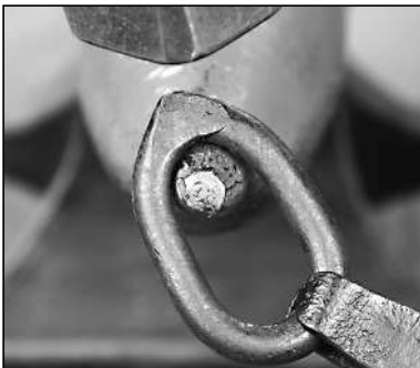
Have the apex tilting towards the heel of the anvil as you work.
