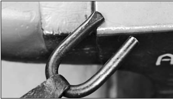
Pivot around the bottom contact point.
