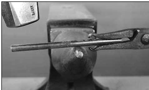
Bend the bar either at the bick or in the pritchel hole.
