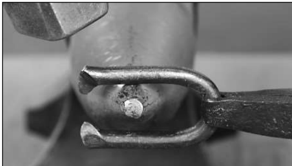
Bend the ends so that they overlap each other.
