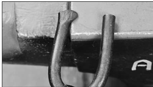
The scarf looks like a flag on the end of the bar.
