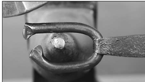
Bend the second arm around the back.
