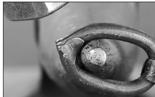
You might need to level the ends so that the points are aligned.
