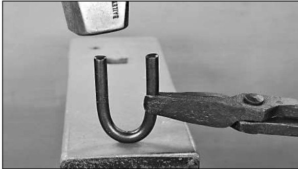
Hammer on the long arm to shorten and close the link.
