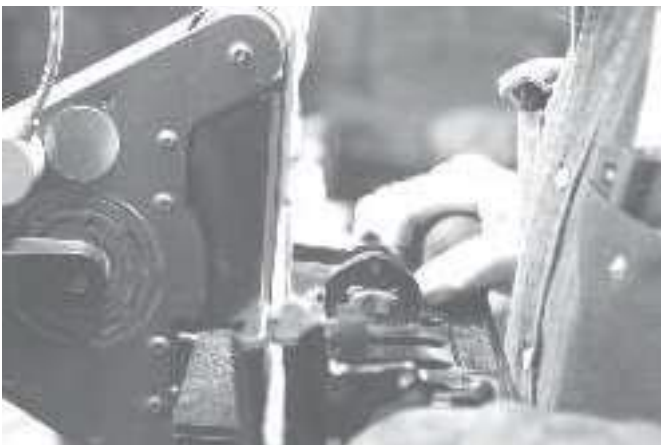
Grinding pass, step 3: Approaching the point, pull the handle end out slightly
