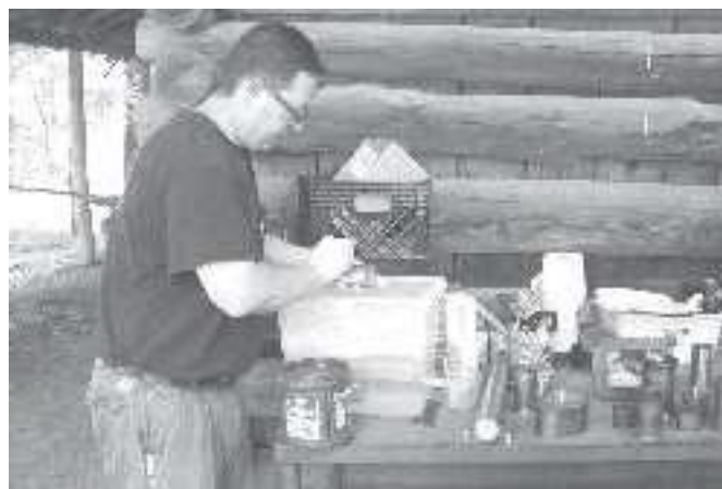
Pickling - soaking in an acid bath - to clean the copper
