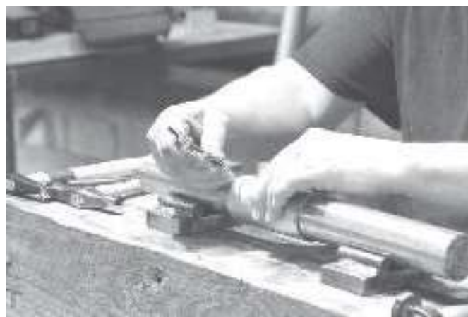
Scribing layout lines around pipe, 1/2 and 5/8 inch from ends
