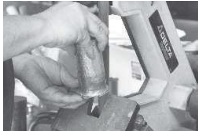
Sand the bottom flush. Copper gets hot - a little water in the cup helps soak up the heat!
