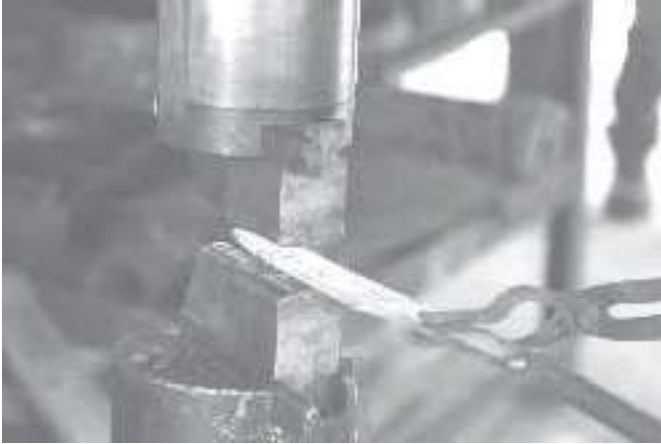
Forging bevels on the power hammer
