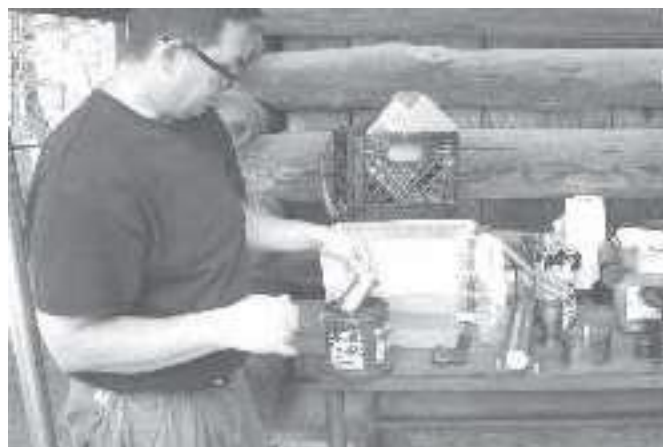
Dipping in liver of sulfur to darken the shiny copper
