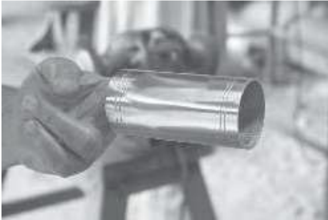
After chasing and then polishing
