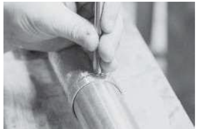
Above: "Stitching" between the chased lines, then...
