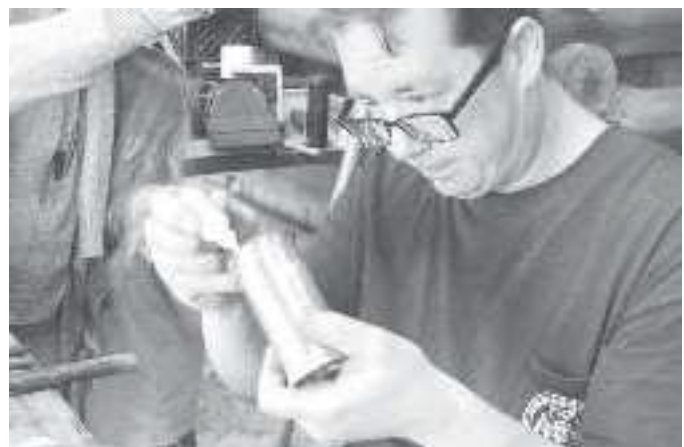
Applying flux to the bottom edge of the pipe
