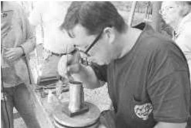
Pushing bits of solder to the joint on the inside of the cup
