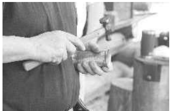
Texture the top edge with another hammer - pick one that makes a nice texture
