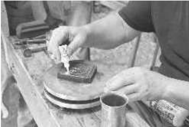
Applying flux around the inside of the Sharpie line on the bottom
