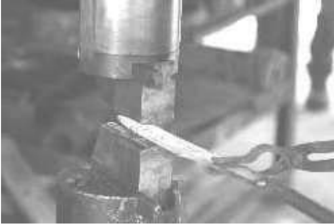
Forging bevels on the power hammer
