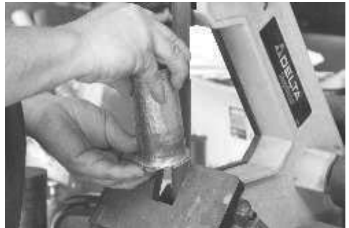
Sand the bottom flush. Copper gets hot - a little water in the cup helps soak up the heat!
