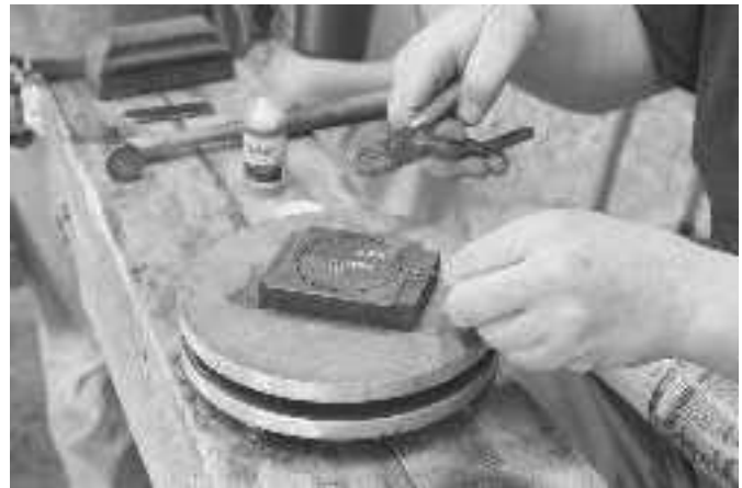
Preparing to solder bottom - trace bottom of pipe with a Sharpie
