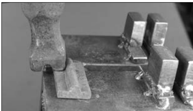
I occasionally use the set hammer on only one side of the collar stock to help true the stock or bend
