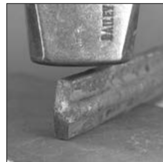
Continue to work in the swage, dressing the edges as you go
