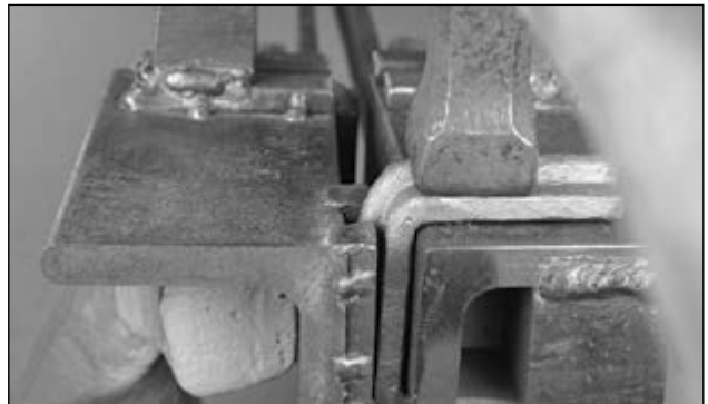
Each bend is made individually. The set hammer is used to clean up the root of the bend point
