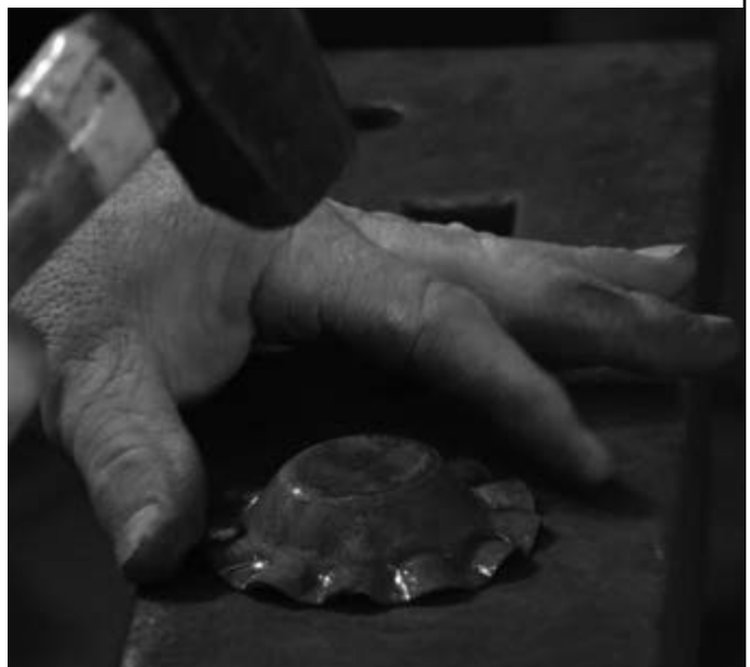
Photo 19: Truing Up the Overall Cup Shape
