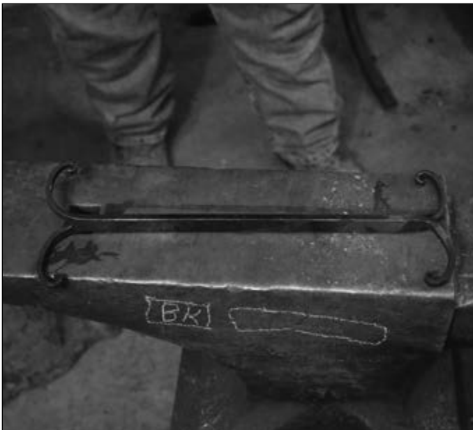
Photo 8: Main Bar Tapered and Scrolled on Both Ends
