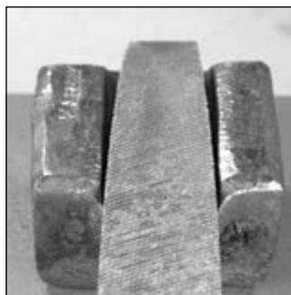
Dress the result, centering the bead and sloping the edges to achieve a mould-release effect and then case harden
