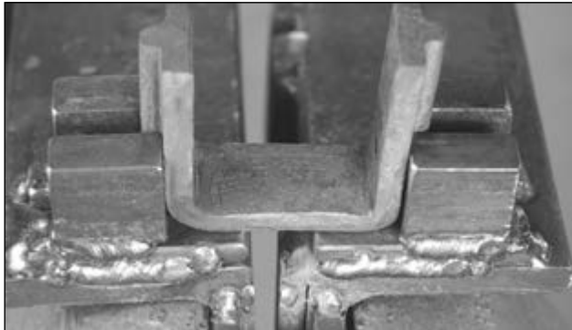
The blocks are to act as a collaring vise. Note the gap between the angle-iron pieces to allow for vise closure
