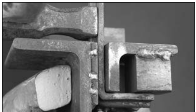
Turn the collar over and bend the second corner using the block as a depth stop for the collar
