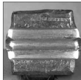
Dress the result, centering the bead and sloping the edges to achieve a mould-release effect and then case harden
