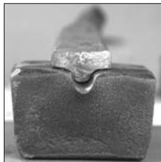
Continue to work in the swage, dressing the edges as you go
