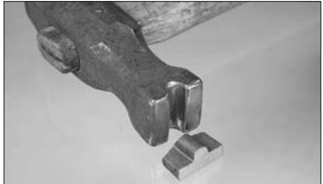
A set hammer with a groove cut into the face to accept the collar bead is also required
