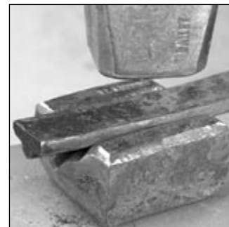
Drive the collar stock into the heated bottom swage to sink in a further depression
