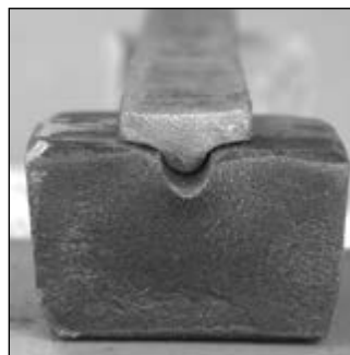
The finished result should be under one-inch wide by whatever thick—with relieved edges at the side of the half-round bead
