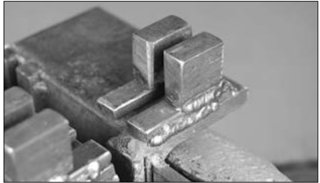
At the other end of the vise inserts, blocks were welded on. Two blocks per side with a \frac{5}{16} " gap between them
