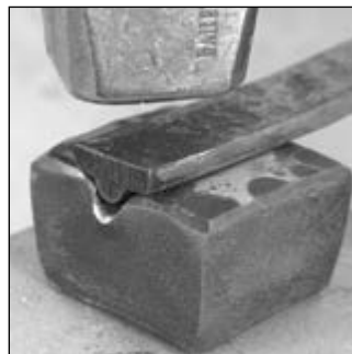
Drive the collar stock into the heated bottom swage to sink in a further depression
