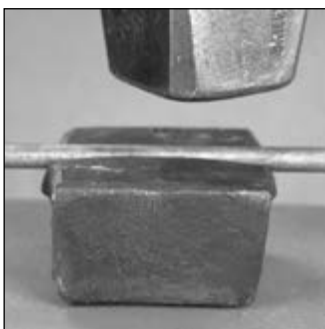
Start at one edge and drive in a 1/4-inch fuller or length of round bar—work to a 1/4-inch depth
