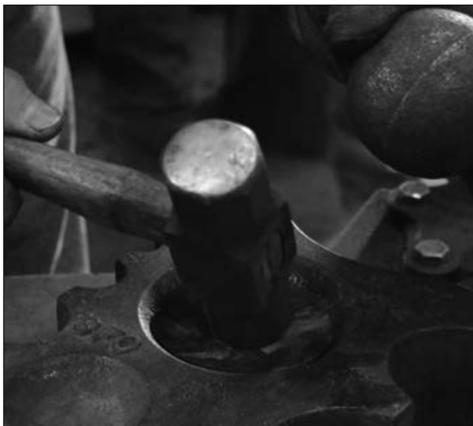
Photo 20: Dishing the Base
