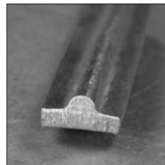
The finished result should be under one-inch wide by whatever thick—with relieved edges at the side of the half-round bead
