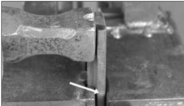
Layout the collar and center punch the edge. Heat the collar and bend using the set hammer
