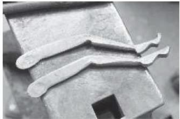
Spread out and round the hinge area. Bend the knee and ankle. File the joint surfaces flat and file any sharp edges.
