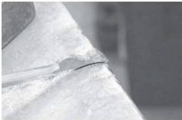
Forge and bend the toes up. "Up" is really down over the edge of the anvil
