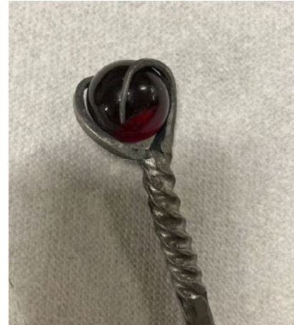
Insert large marble in cold stock using long nose vise grips or pliers.
