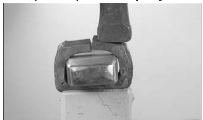
Dressing the rear corners, note that I need to cut more of the ends away before they interfere with each other.
