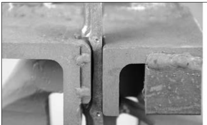
The collar material with the center punch mark held 1/8" (half the thickness) above the surface of the bending jig
