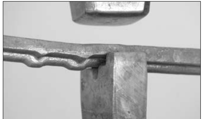
Move corner #2 out from the offside edge and extend the forging between the corners #2 & what will be #3
