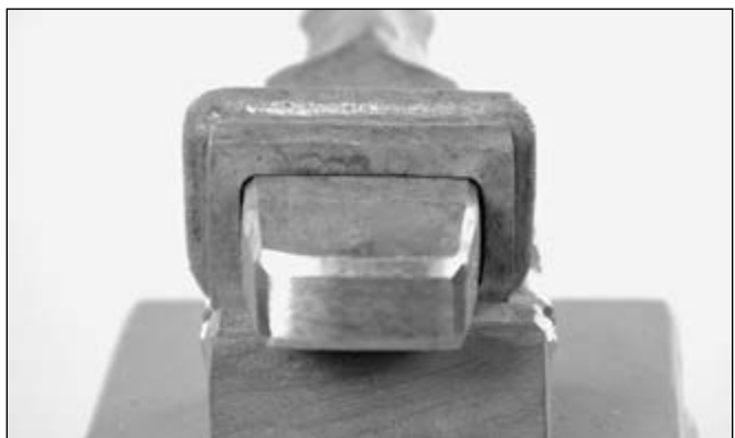
A look at the front of the collar after rasping the edges at the vise
