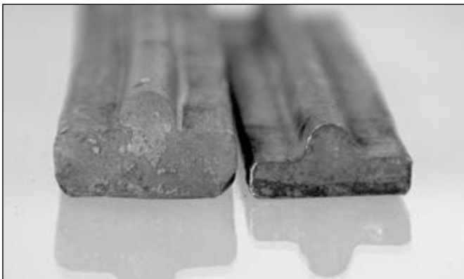
A comparison of the two different collar stock sections. Left, intended for the forged collar, Right for a wrap collar
