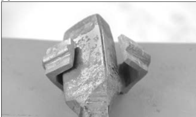
Check that the mandrel will fit in through the opening. If the mandrel fits, so will the grille
