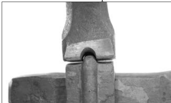
The top tool fits the bead but doesn't touch the back-strap, allowing for the bead to be forged
