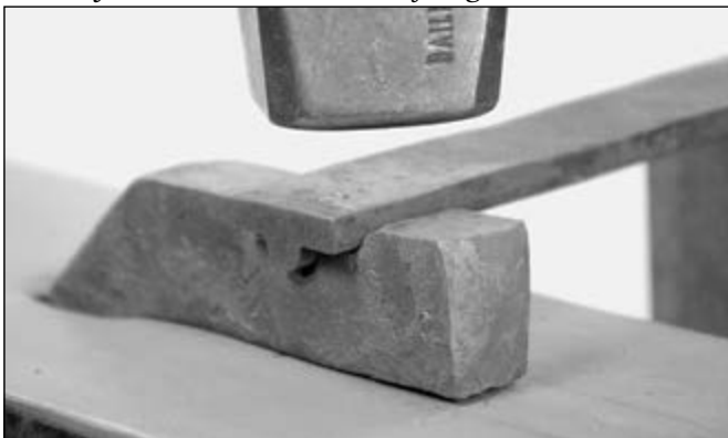
Continue to drive the collar material down, until the back of the bar is level with the top of the swage
