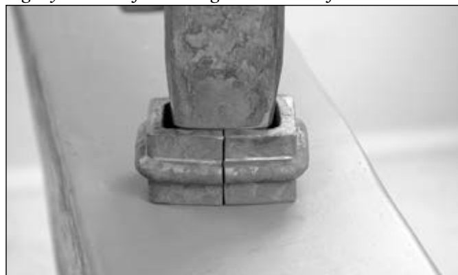
The taper should be sufficiently long so that the collar falls off the end of the mandrel
