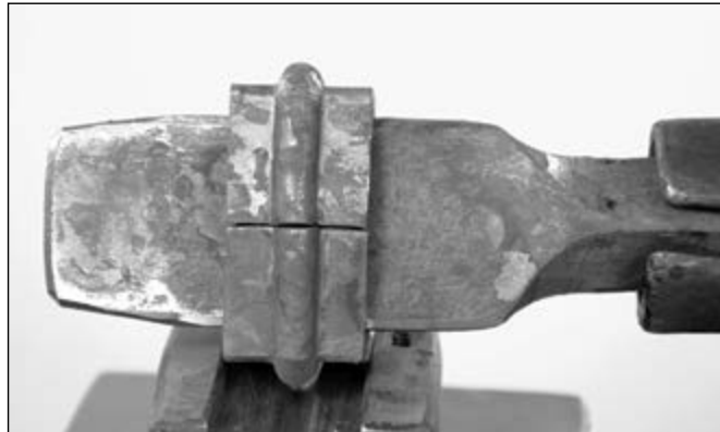
If you use the collar material swage as a backing, the collar will get pinched between the edges as it spreads
