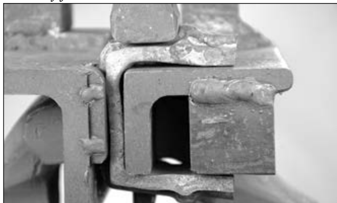
Dressing the second bend using the top tool
