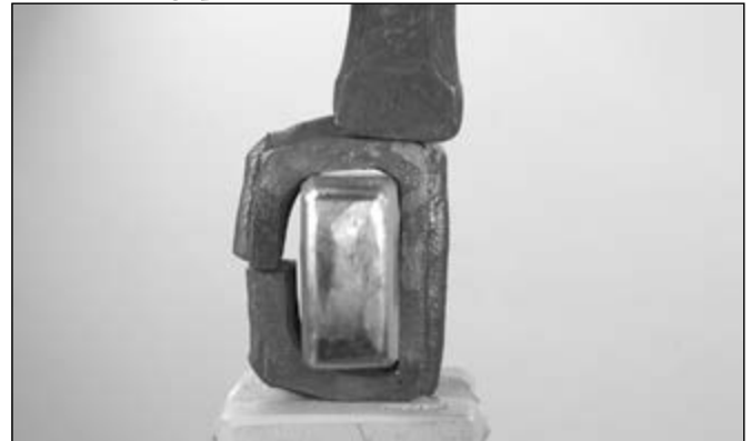
I like to work the corners on what will be the front of the collar first. Some of the work is an upsetting action
