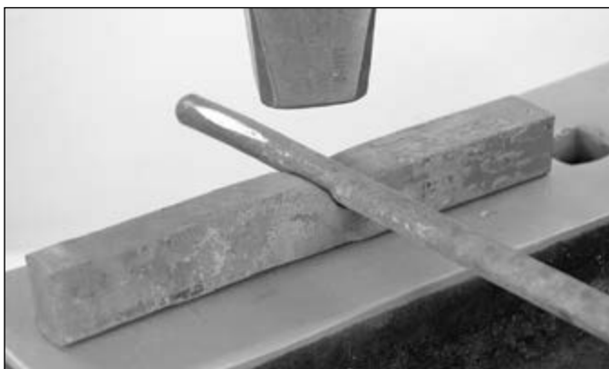
Drive a fuller in at just below the transition area
