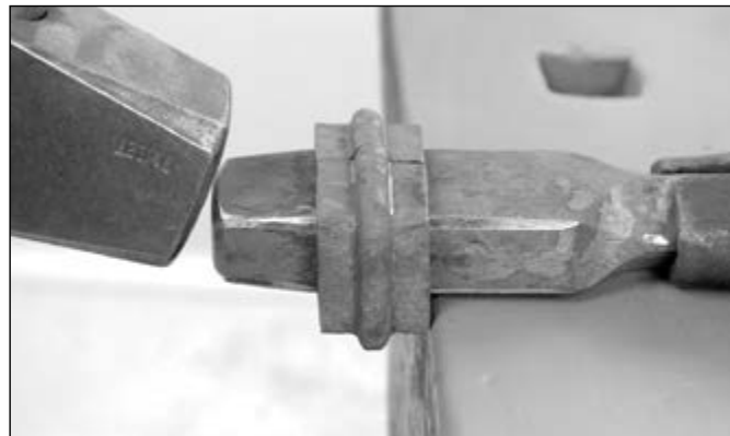
The mandrel has a compound taper at the tip, and is slightly crowned facilitating the removal of the collar
