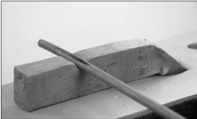
Use a 1/4" rod to start the depression for the collar material. I find that the rod helps square the depression
