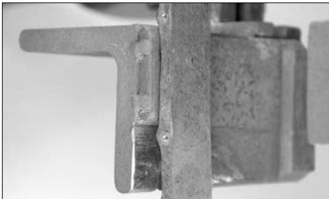
The collar material held against one side of the bending jig. Note the room for the corner material
