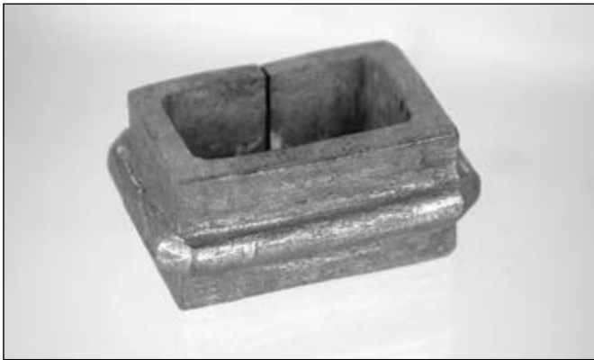
A forged collar ready to be opened and hot fitted to the grille.
