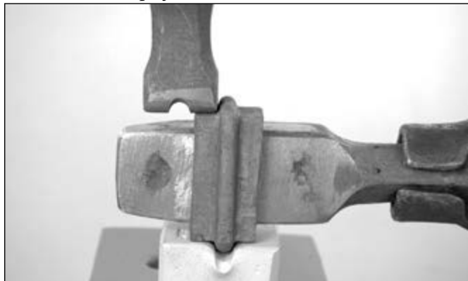
You will sometimes use the top tool on one side of the bead or the other as you work up the collar
