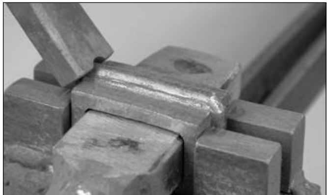
With the collar supported in the bending jig, and using a dedicated tool, dress the corners of the collar
