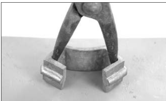
Use scrolling tongs to open the collar, don't open the gap much more than 1-inch, as it's hard to close later.
