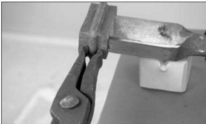
I find that using rivet tongs are helpful when working with the collar. The ability to grab the bead can be key
