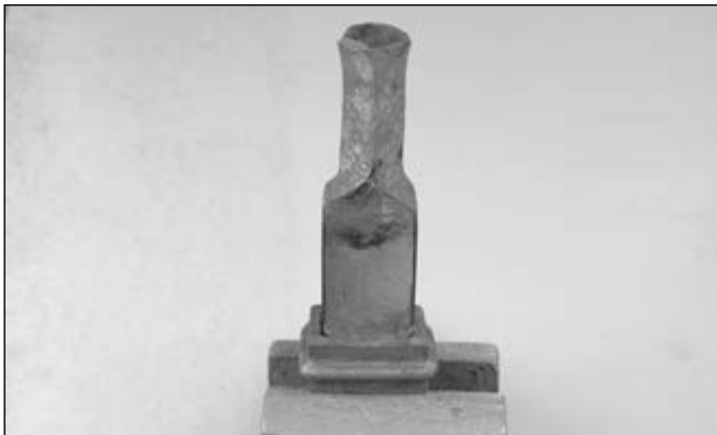
Fitting the collar to the mandrel at the vise. My tongs [usually fitted] have been removed for clarity
