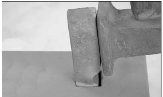
Place the square bar into your hardy hole, forging to suit if required
