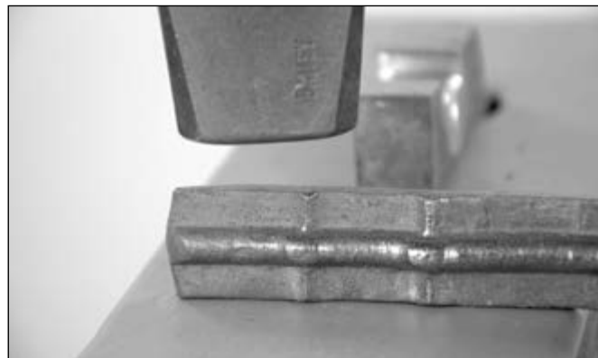
Dress the sides of the collar material as you work in the swage
