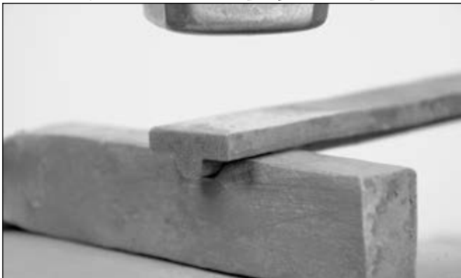
Follow with some forged collar material. Reducing the width of the material will aid in filing to size later
