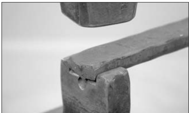
Match the end of the bar to the offside edge of the swage, and drive the material down
