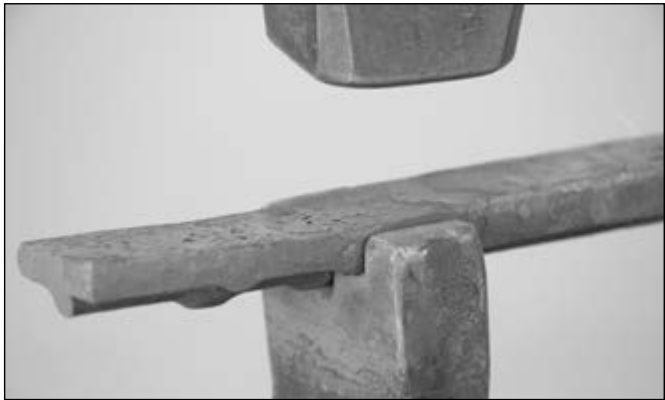
Drive in the collar material, finishing corner #2
