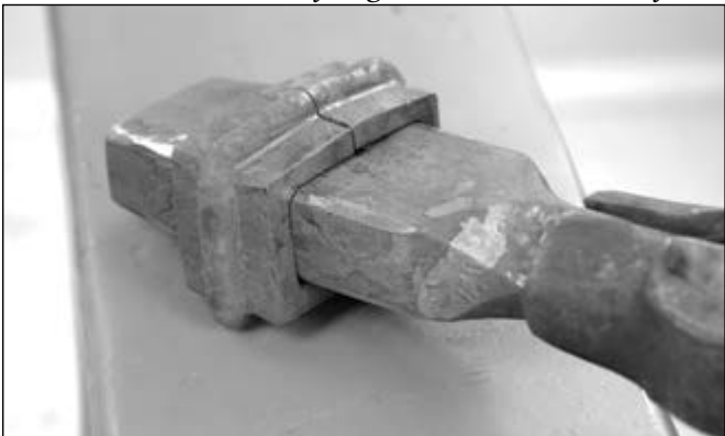
In this case the ends are interfering with each other before the corners are finished. Cut another gap
