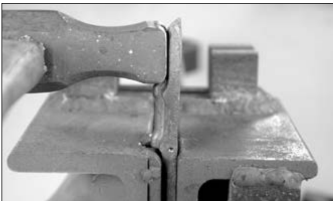
The center-punch mark is held half the thickness of the collar above the bending jig
