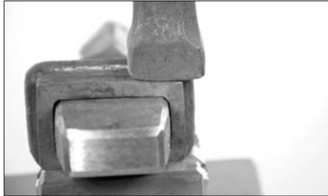
The top tool helps form the corners of both the bead and the back-strap of the collar
