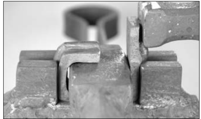
I don't usually meet a lot of success making this bend unless I change position or turn the collar around
