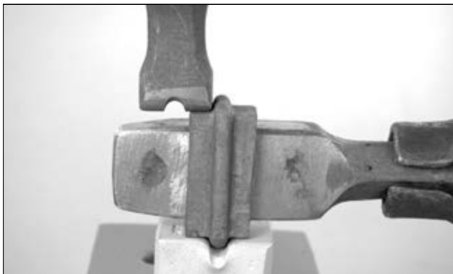
Working on the offside edge of the back-strap with the top tool.
