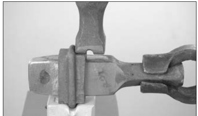
Working the nearside edge. The edges of the tool are relieved to match the bead to back-strap transition
