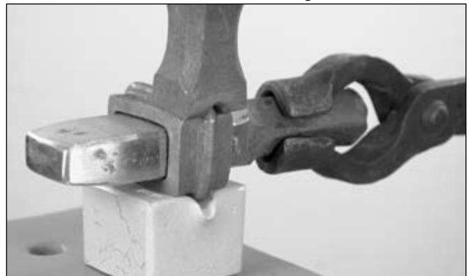
This is the collar shown on the previous page taking shape. This is the end of the second heat
