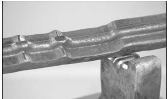
The forging for what will be the front of the collar, which requires a greater distance between the corners
