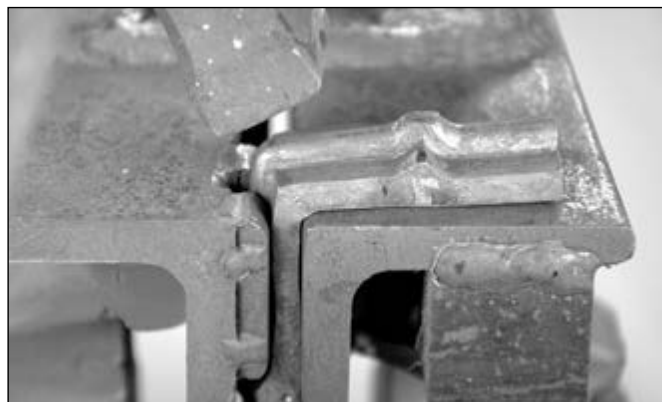
The jig forces the excess corner material out almost forming the square corner on the back-strap
