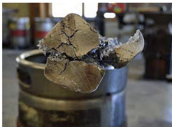
Figure 3: 3" Aluminum rod forged at too high a temperature
