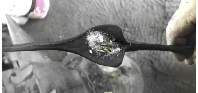
15. Insert the shavings and borax flux for brazing, Make sure to keep upright so that the shavings don't fall back out!
