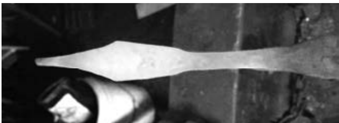
3. Make a nice concave taper on the end. Make the necked-down section parallel.
