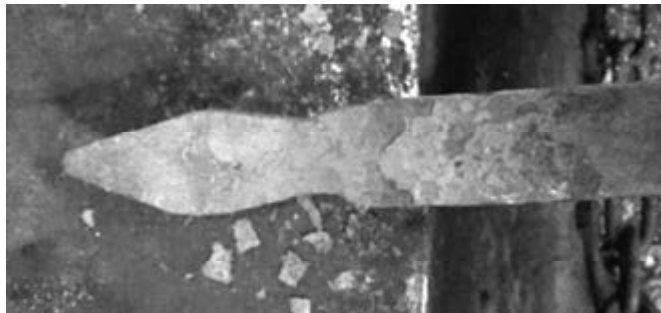
1. Taper the tip, and make a neck centered about 1 1/2" back from the tip. Maintain thickness at 1/4".
