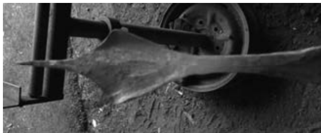
5. Spread the "wings" more. Make the transition (left edge in above picture) concave.
