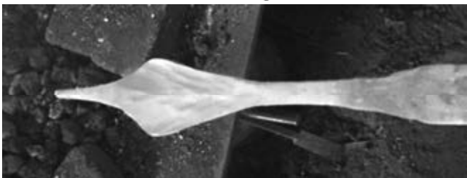
4. Use the cross peen to spread and thin the center section.
