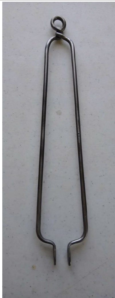
Above: Completed coal tongs. This project includes many basic blacksmith skills such as: upsetting, twisting, centering, bending, measuring and adjusting. Perfect for demonstrations and beginning projects.
