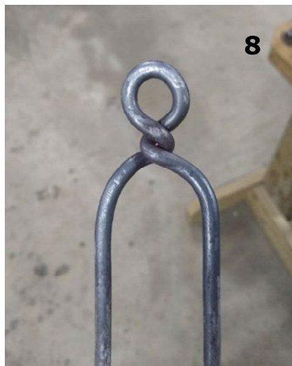
Above: Completed coal tongs. This project includes many basic blacksmith skills such as: upsetting, twisting, centering, bending, measuring and adjusting. Perfect for demonstrations and beginning projects.
