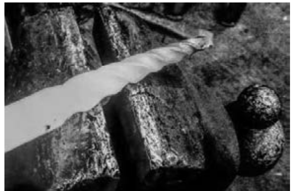
Twist the taper in several sections as shown by arrows.
