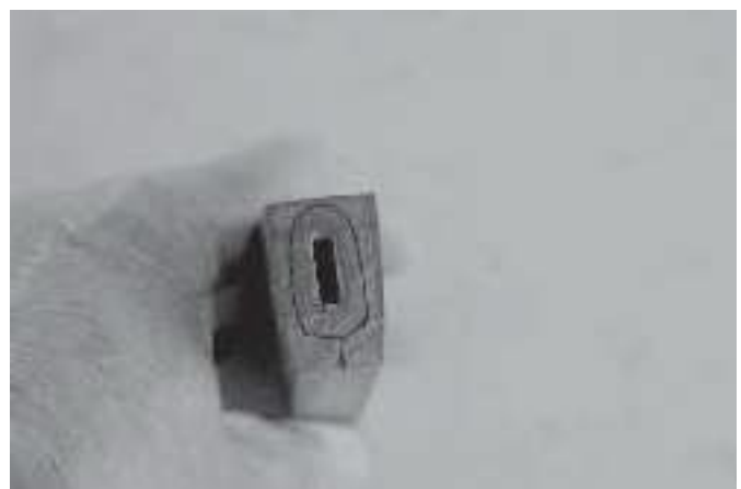
Draw the outline of the guard and the handle on the block, then grind the block separate from the blade.
